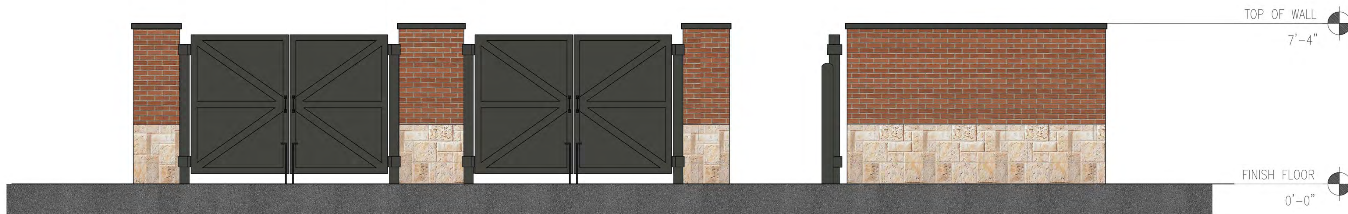
5 ELEVATION - DUMPSTER ENCLOSURE 3/8" = 1'- 0"
